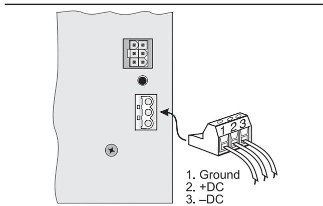
Figure 1. Model 732A cabinet showing 3-position plug-in terminal strip
