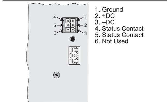
Figure 2. Model 732A cabinet showing 6-position connector
