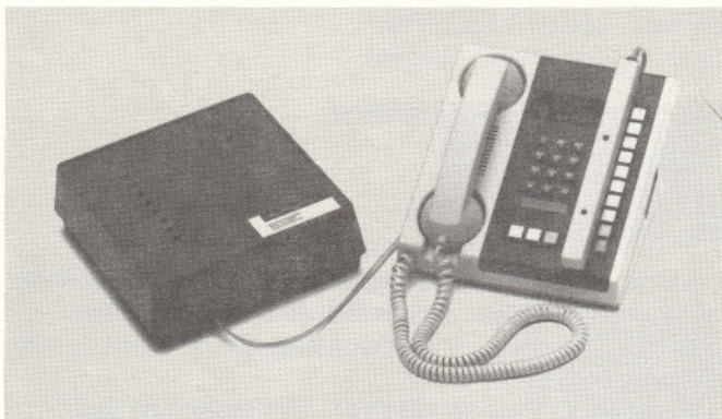
Figure 1 Model 301, main unit with sensor assembly attached to the telephone.
