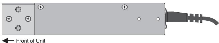
Figure 5-3. Model 135 Side View Shown with Mounting Brackets Attached for Wall Mounting
