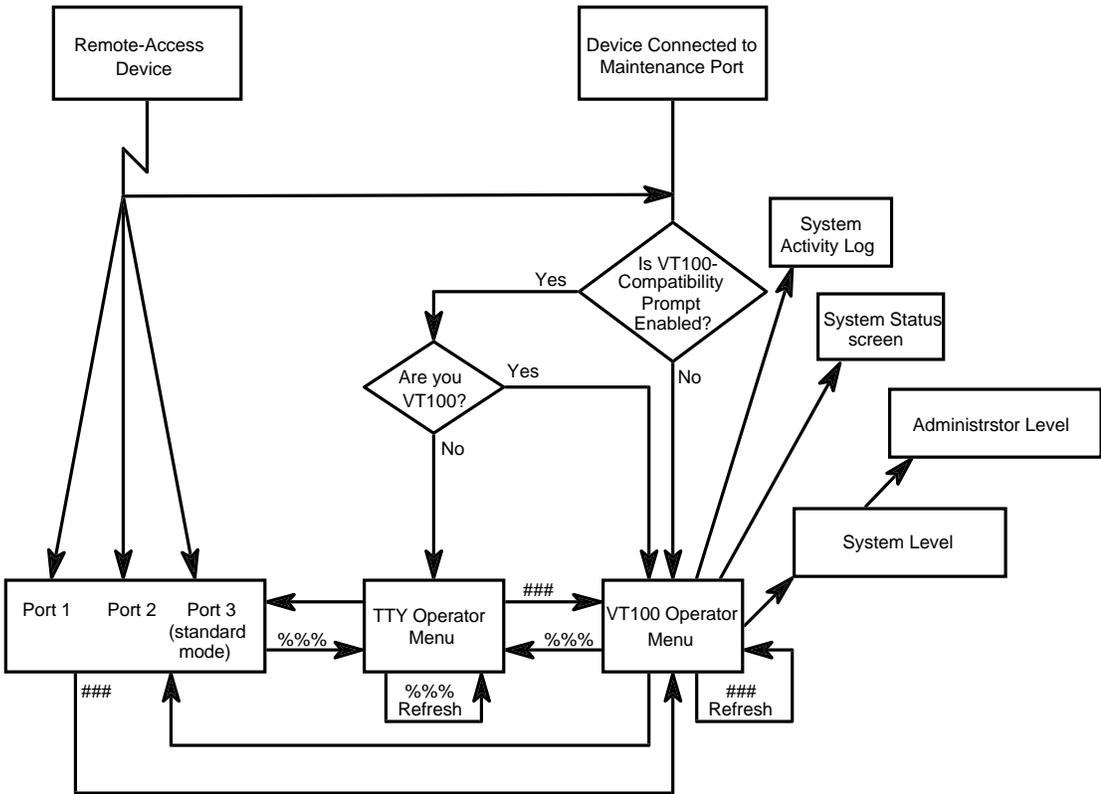
Figure 14-4. Model 125 Operator Menu Access
