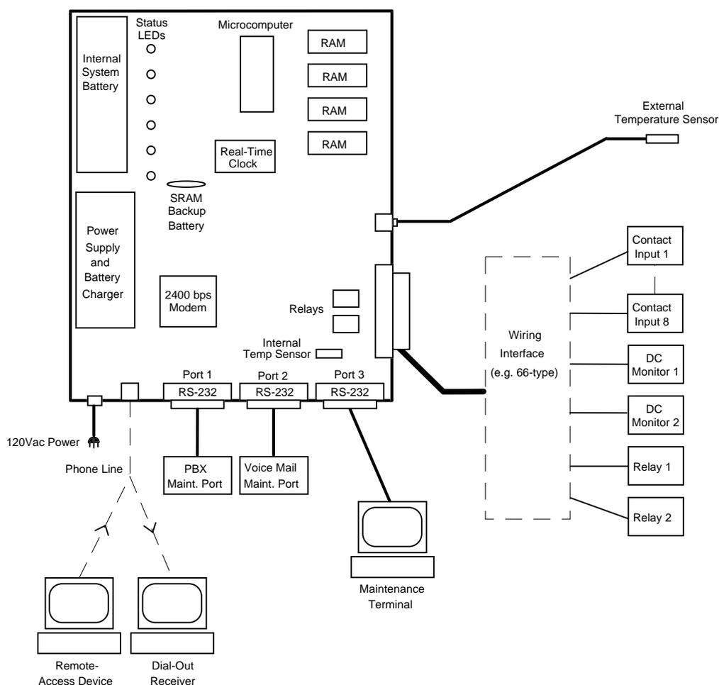
Figure 1-1. Model 125 Installed in a Typical PBX-System Site
