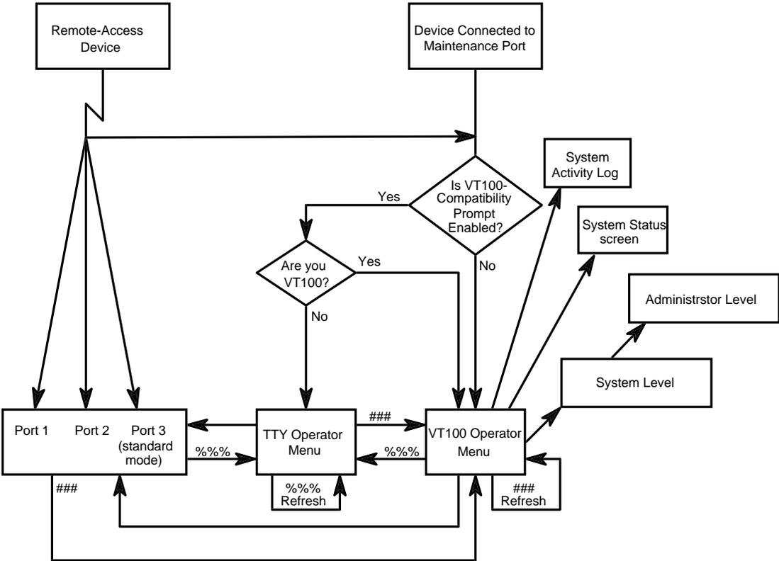
Figure 14-4. Model 125 Operator Menu Access
